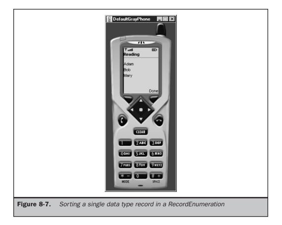
The next change occurs in the third try {} block where an instance of the RecordComparator() interface is created and passed as the second argument to the enumerateRecords() method. A null was passed as the second parameter to the enumerateRecords() method in Listing 8-7 because the RecordEnumeration was not sorted.
