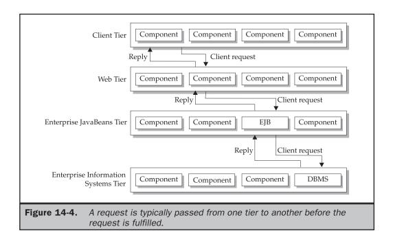
that are called upon indirectly by clients. The EJB Tier is the keystone to every application because Enterprise JavaBeans working on this tier enable multiple instances of an application to access business logic and data concurrently so as not to impede performance.
