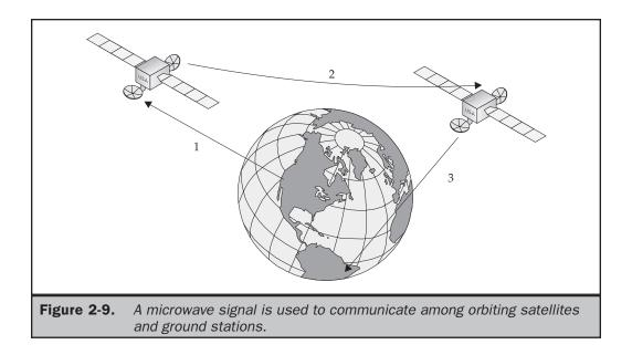
covered by geosynchronous satellites. The other problem is the orbital speed. LEOS travels faster than the earth's rotation and requires ground stations to locate LEOS before beginning transmission. Geosynchronous satellites always remain in the same position above the ground station.
