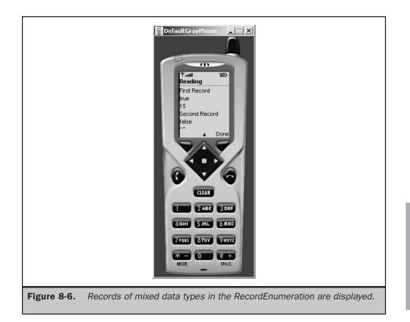
The readUTF() method, readBoolean() method, and readInt() method are then called to return their respective data from the current record of the RecordEnumeration. These return values are then concatenated and assigned to a string. The string is then displayed in an alert dialog box (Figure 8-6). The same process occurs for each record in the RecordEnumeration.
