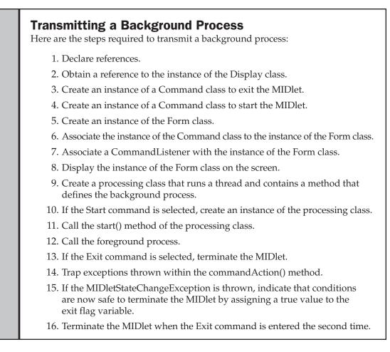
The Process class defines the start() method. The start() method creates a thread and then calls the start() method to run the thread. The run() method calls the transmit() method. The transmit() method contains all the code to send or receive a transmission.
