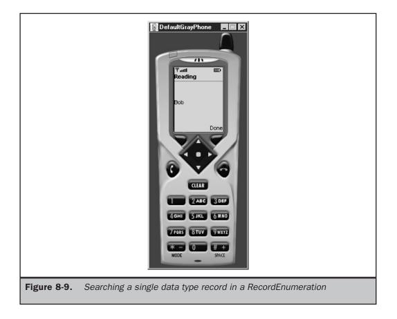
The statement beneath the statement that created the instance of the Filter creates the RecordEnumeration. The enumerateRecords() method is passed three parameters. The first is reference to the filter. The second is reference to the Comparator. This is set to null because a Comparator isn't used in this example. The last parameter is a boolean value indicating that the RecordEnumeration should not be automatically updated when changes are made to the underlying record store.
