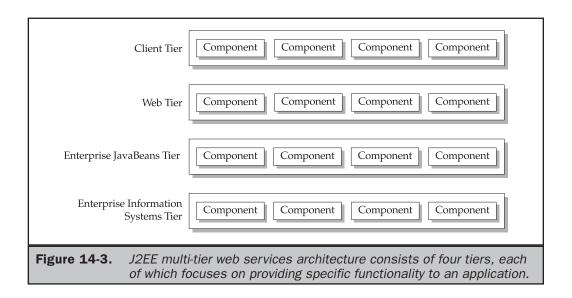
web services architecture is functionality-centric, an application accesses only tiers whose functionality it requires. It is also important to disassociate a J2EE API from a particular tier. That is, some APIs (XML API, for example) and J2EE components can be used on more than one tier, while others (Enterprise JavaBeans API, for example) are associated with a particular tier.
