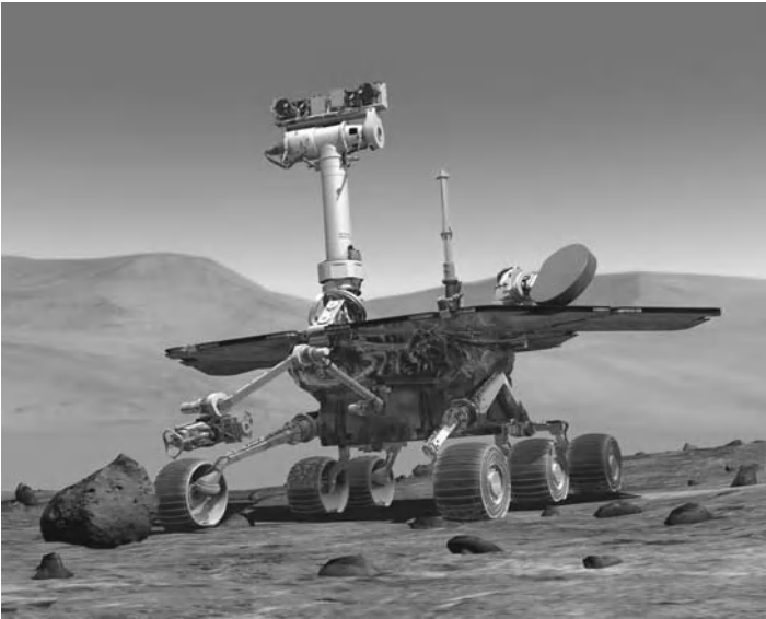
Figure 1.6. Mars Exploration Rover; a solar-powered, autonomous real-time system with radio-communications links and a variety of sensors and actuators. Photo courtesy of NASA.
